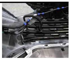
NOTE: holes in bumper may need to be enlarged to allow harness to feed through.
